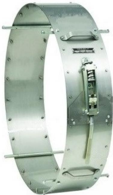
Hand- or electric powered band crawler type pipe-cutting machine, available for pipe sizes 6" and larger.
