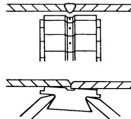
The conical fingers operate independently from each other, by this pipes are always clamped "in line".
