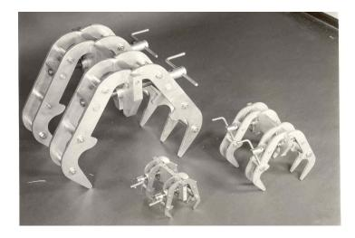
The Centromat external centering tools are deliverable in three measure ranges :
