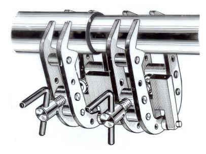
The CENTROMAT external centering tools are ideal tools for clamping and centering pipe/pipe connections. If there is a difference in pipe diameters and these diameters are within the minimum and maximum range of our equipment, the differences are evenly divided over the circumference so that the center lines are always in one straight line.
