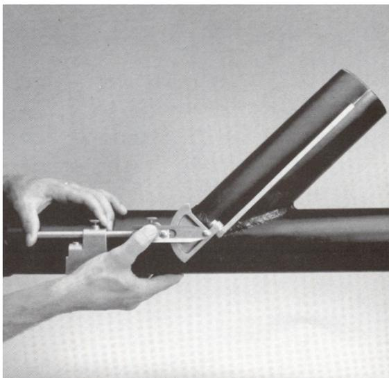
No. 9 **Fitter-Welder Protractor**
