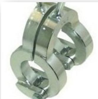
When using this clamp, tack-welding is not required. Simply complete the root pass and then remove the clamp.
