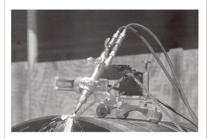
The H&M motorized beveling head is constructed of cast aluminium. It is lightweight, compact design allows for easy one-man setup and operation. Seventeen different stainless steel bands provide a cutting range of 10" to 96' diameter pipe, plus special bands are available for cutting pipe up to 20 feet in diameter.
