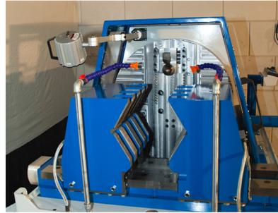
The copying system can be fitted to existing machines (PBM-16 or PBM-30). The original tool head is replaced in that case by a tool head with the copying system that is mounted directly on the main shaft.
