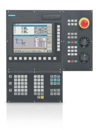
The newest developement is to execute these two models with a CNC-control. The consequence of this is that the machine will have an easy to operate screen. In this screen you can choose the bevel form you want to make (e.g. V-J-compound form). Then you fill in your dimensions and the machining is done automatically.
