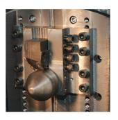
The copying system can be fitted to existing machines (PBM-16 or PBM-30). The original tool head is replaced in that case by a tool head with the copying system that is mounted directly on the main shaft.
