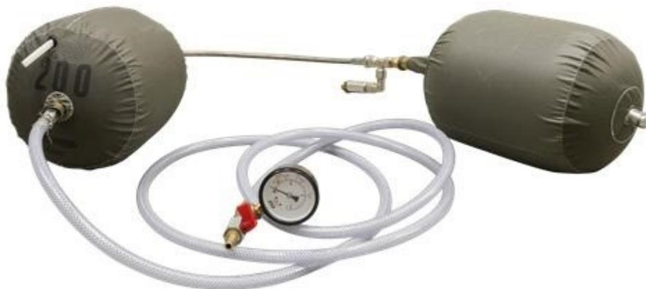
This Backing gas system consists of two closing bladders (up to 70° C).
