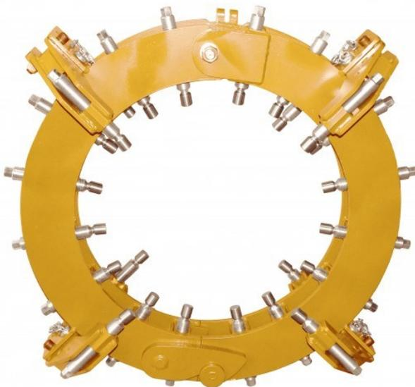
The RIM and ULTRA RIM Clamp series are designed to take on some of the toughest reforming jobs in the industry. These clamps make easy work of aligning and reforming. The standard RIM clamp is capable of reforming X45 - Sched. 80 with out-of-round conditions up to 50 mm. (depending of the pipe diameter).
