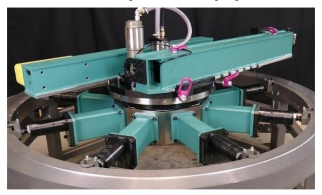
With the TFD Flange Facers, damaged or distorted flange surfaces can be easily cleaned up. Depending on the operation (turning or milling or grinding) one can select all values of surface roughnesses.
