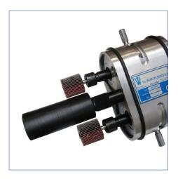
The replaceable flap wheels are available in diameters 30 and 50 mm. The (black) strip wheels are available 50 mm only. The polishing width is 30 mm for the flap wheels and 25 mm for the (black) strip wheels.
