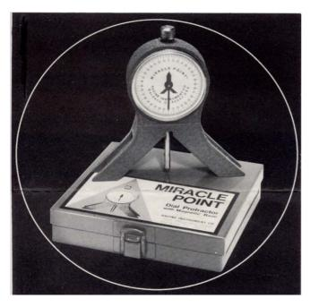
The Miracle Point Model 345-10 Dial Protractor is a 360° angle finding, center locating and leveling instrument reading directly from 0° to 90° in any position with accuracy to three minutes of a degree.
