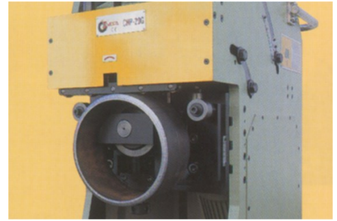
Pipe ends beveling from 150 mm. I.D.
