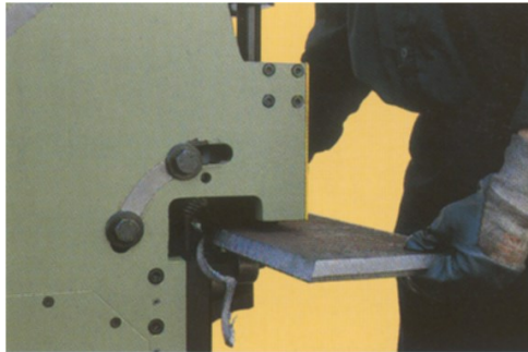
Small sheet pieces can be inserted manual.
