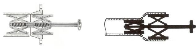
The Centromat tools are designed for clamping and centering a flange to a pipe (also for slip-on flanges). The tools are available in the range from 16 to 950 mm. I.D. and made of steel or stainless steel. It does not matter when the two internal diameters are different (see picture right at the top) the tool will always align the both pieces.
