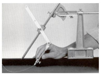
No. 14 **Circle-Ellipse Projector** for marking off circles and ellipses on pipes, tanks, boilers etc. A strong magnetic foot keeps the projector on his place.
