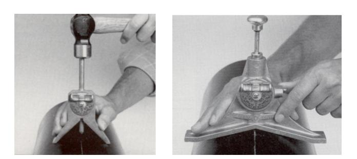
**Centering heads** are available in 2 types. Type Jumbo is provided with an automatic centering punch.
