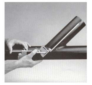
No. 9 Fitter-Welder Protractor Ruler length 300mm.
