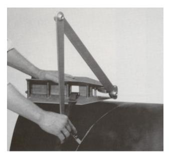
**Contour markers** for marking off **pipes and structures** as T and Y connections:
